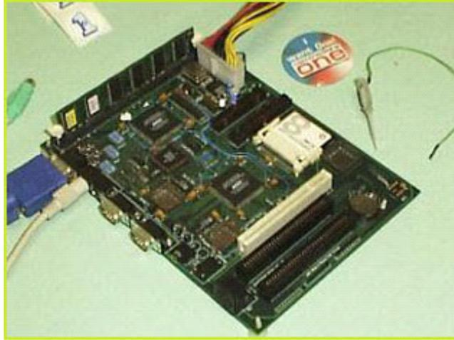
Jakub's ARM board as a replacement for the PIC chip. However, Tobias' implementation uses a different approach: A second instance of the 68000 processor replaces the ARM processor. This makes the C-One with FPGA extender the best-equipped Minimig on the market!
