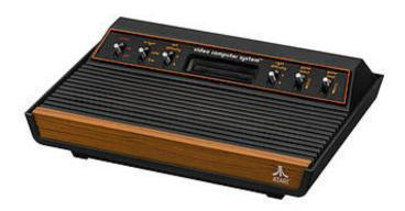
The second 2600 model is the "Light Sixer" which has lighter plastic molding and shielding than the 1977 launch model.
