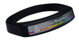
The Atari Mindlink is an unreleased video game controller for the Atari 2600, originally intended for release in 1984. The Mindlink was unique in that its headband form factor controls the game by reading the myoneural signal voltage from the player's forehead. The player's forehead movements are read by infrared sensors and transferred as movement in the game.
