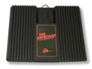
The full name for this was The Joyboard Power Body Controller. It's a large, flat, black board with red lettering that users stand on to control their games. By rocking back and forth and side-to-side, they simulate the joystick motions. An additional port in the Joyboard allows them to plug in a stick for use with games that need a button. It was packaged with the game, Mogul Maniac.
