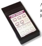
Also known as the Star Raiders controller, functionally identical to the Kid's Controller and Keyboard Controller. Game included an overlay with commands, for use with Star Raiders.
