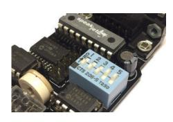
Also onboard the AtariVox+ is 32K of non-volatile memory which can be used as a memory card. The flash memory will retain data without power for 200+ years.
