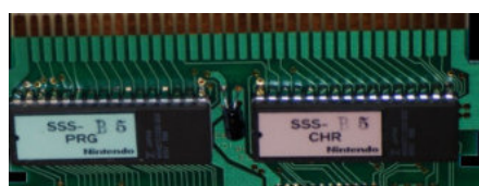
Official Nintendo TKEPROM Prototype Board with Official Nintendo Prototype Stickers
