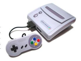
The Super Famicom Jr. was lighter and more compact redesign of the original Super Famicom console. It was almost identical to the SNS-101 console released in North America previously, and featured the same connections and outputs.
