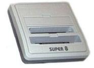
The Super 8 (also sold under the title Tri-star) was an unlicensed peripheral designed to allow the system to run games developed for the NES and Famicom. The Super 8 utilized an NES-on-a-chip (NOAC) integrated circuit to duplicate the functionality of the original NES hardware, and connected to the SNES's own cartridge port.
