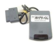
The Voicer-kun (sometimes erroneously called "Voice-kun") from Koei is an infrared transmitter/receiver for the Super Famicom that connects to the second controller port. The IR-transmitter is used for controlling Audio CD players, and is able to "learn" IR-signals from different CD Player manufacturers.
